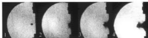
(a) Brick target, impact velocity = 322 m/s, interframe = 300 μs.
