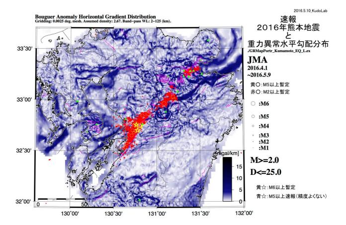
Relationship between fault structures detected from gravity anomalies and the aftershock distribution of the 2016 Kumamoto earthquake
