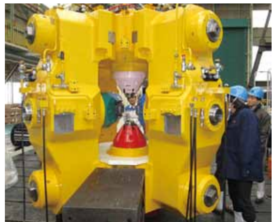
The multi-anvil high pressure apparatus installed in a neutron beamline of J-PARC (Image courtesy of Dr. Takehiko YAGI)
