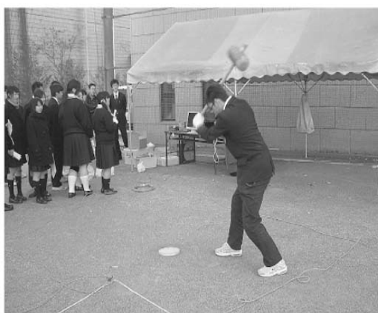
Fig.1 Photo of the experiment. The student is generating seismic wave by using wooden hammer.
