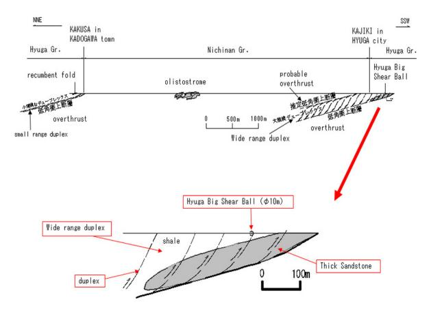
The Shear-balls in Miyazaki Prefecture are existenced in the fracture zone near the large-scale thust in Shimanto Terrain.
