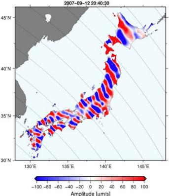
a broad band seismic record by applying simulation filter to the observed seismogram (e.g., Kanamori et al., 1999). This is a second-order, recursive time domain filter; we can recover broadband signal with relatively small computational cost.
