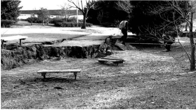
Photo: Fault (approximately 190m in length and approximately 70cm in throw; open sense) in liquefied zone at Hamigawa-ryokuchi, 3 Utase Mihama-ku Chiba city, Chiba pref.
