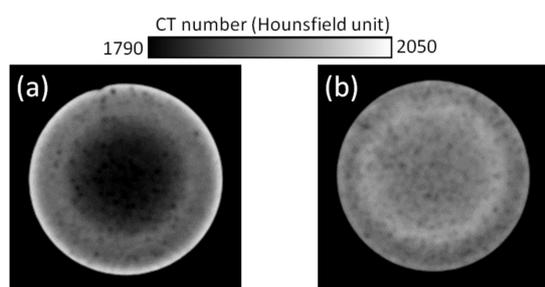
Fig. 1. Two-dimensional CT slices of homogeneous sand pack samples (diameter, 56 mm) saturated with a heavy-element-bearing fluid. Each image dimension is  $210^2$  voxels =  $66^2$  mm<sup>2</sup>. The image for KI 9.16 wt.% (a) shows marked beam hardening compared with  $\text{Na}_6\text{H}_2\text{W}_{12}\text{O}_{40}$  8.80 wt.% (b). Numerous dark spots are small bubbles.
