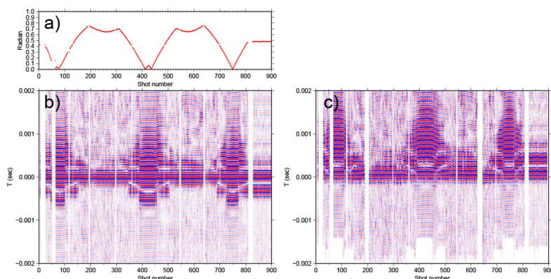
Fig. Incident angle of transmitted signals (a). Pasted correlation waveforms analyzed by reading maximum peak (b) and reading iteratively-deconvolved peak (c). Each trace was moved out by the observed traveltine.
