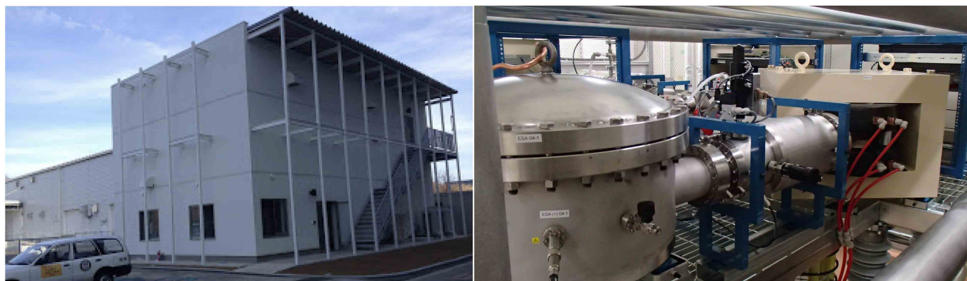
AMS building (left) and Single Stage Accelerator Mass Spectrometer (right)
