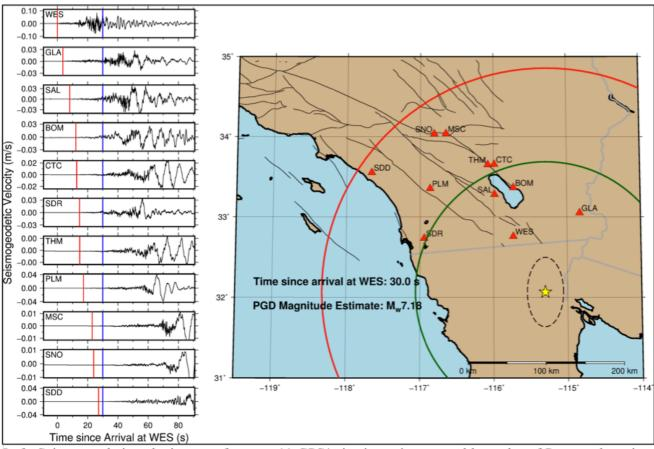
Left: Seismogeodetic velocity waveforms at 11 GPS/seismic stations sorted by order of P-wave detection. Continuous blue vertical line denotes current epoch. Preceding red lines indicate when P-wave was detected from seismogeodetic velocity at each station.
