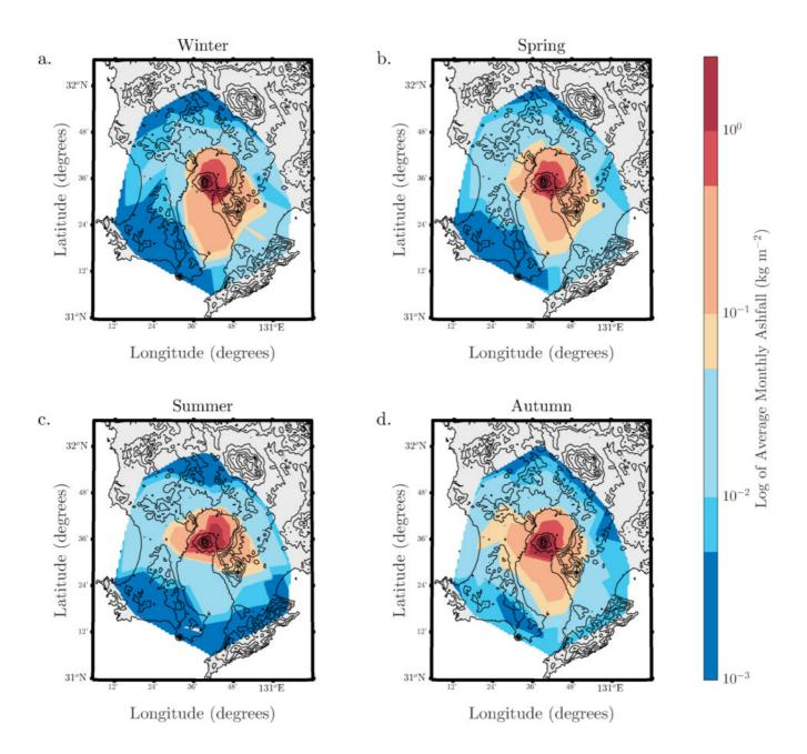
Reinterpretation of wind effects on volcanic ash transport process with Hoei eruption of Mt Fuji by using unsteady numerical simulation
