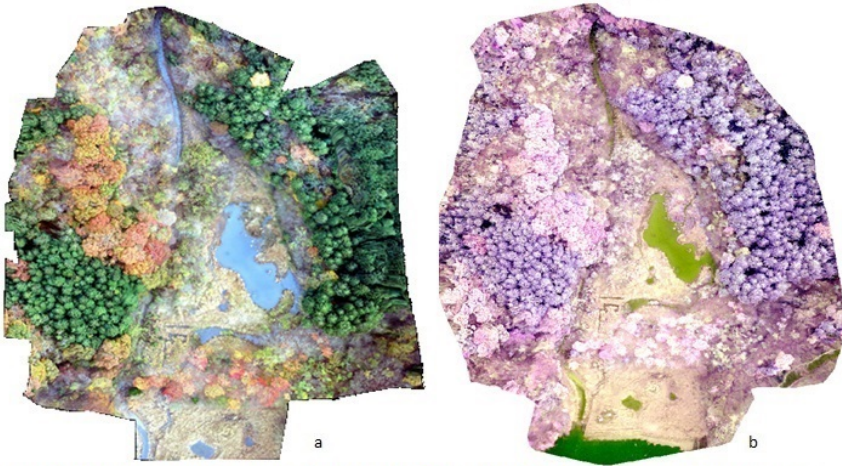
Fig.1 UAV photo result; a) optical image (RGB=123) and b) NIR image (RGB=NIR:R:G). Cooperation with Sagami River Water System Wide Area Dam Administration Office, Ministry of Land, Infrastructure, Transport and Tourism.
