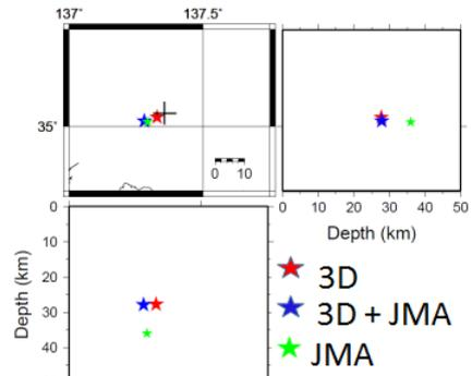
**Fig. 2.** An example of the difference in depth of hypocenter of LFE (LFE13) between 3D, 3D+JMA, and JMA. The 3D and 3D+JMA hypocenters were located using not only S-arrival times but also P-arrival times, while the JMA hypocenter was located using only S-arrival times.
