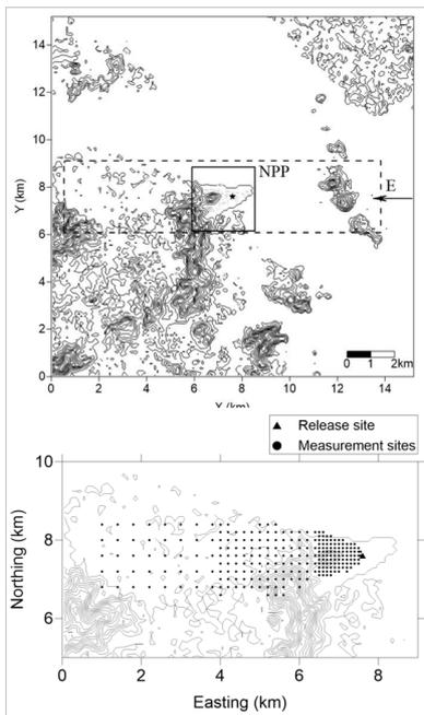
Fig. 1 Topography and measurement network of the wind tunnel experiment
