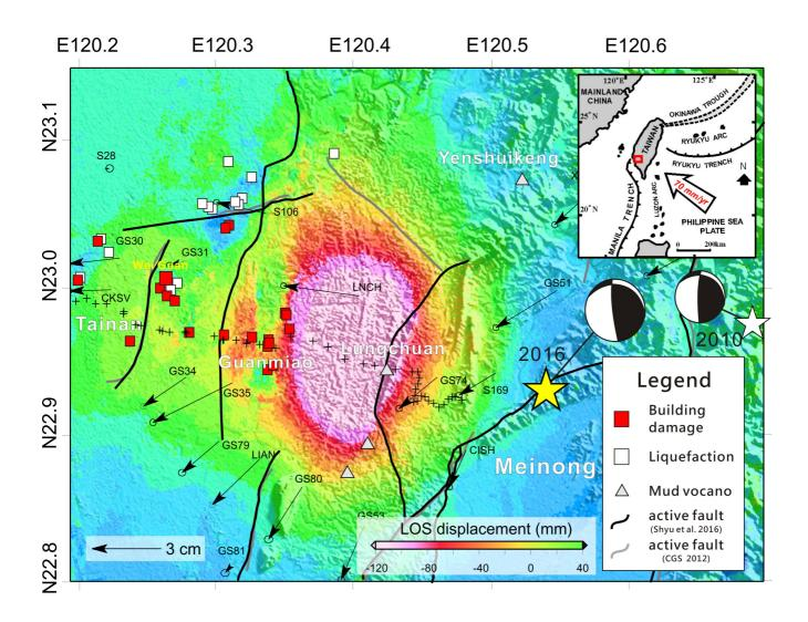
SAR干渉画像に現れた阿蘇外輪山北西部の地表変位の現地検証とその解釈 Field survey and interpretation of the surface linear ruptures in northwest of the outer rim of the Aso caldera emerged on SAR interferogram
