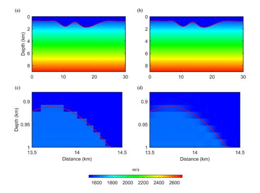
An acoustic velocity model containing an undulating seabed, sampled using the (a) Integral Grid Model and (b) Fractional Grid Model methods. (c) and (d) are enlarged views of the areas outlined by the red dotted squares in (a) and (b), respectively. The red curve in each panel indicates the true position of the seabed.
